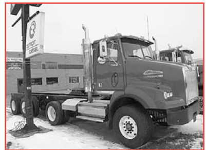
NEW - 2010 WESTERN STAR 4900SA STRAIGHT TRUCK (CAB AND CHASSIS) MERCEDES ENG; MBE4000, 410 HP, 8LL TRANS; 20 & 46 W/PUSHER AXLE(S), 276" WHEELBASE. -51791
